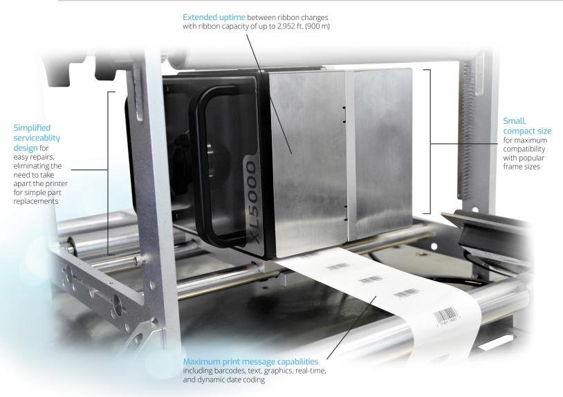
The Allen XL5000 thermal transfer printer is an industrial workhorse that pairs perfectly with most consumer-packaged goods web and foil printing applications. The small, compact size and simplified serviceability design makes it easy to integrate with labeling and packaging machines. The Allen XL5000 is available in continuous and intermittent modes, with a wide variety of dynamic print message capabilities.
